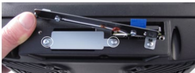
Fig. 15-5: Screws from the battery cover
