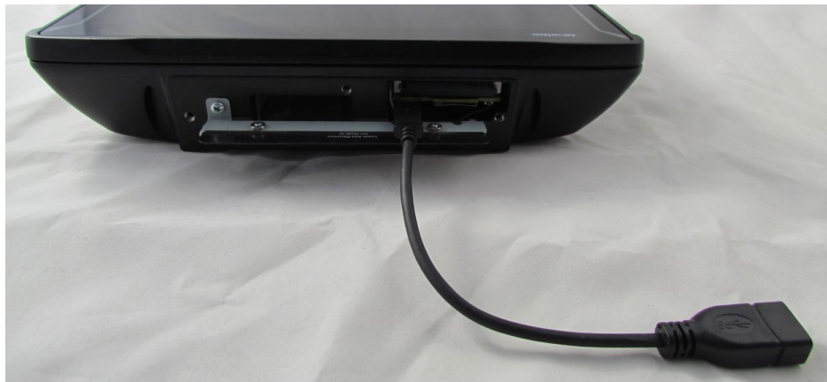
Fig. 7-25: Connected adapter to USB Type-C Service Port (with Taiwan Anjie Electronics antenna)
