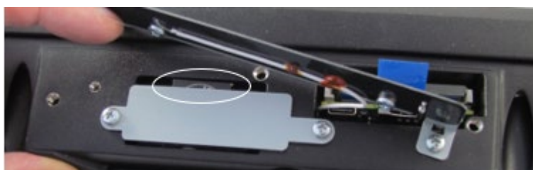
Fig. 15-8: Removal tab under the battery cover
