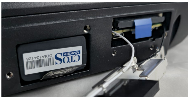
Fig. 15-12: Inserted battery pack
