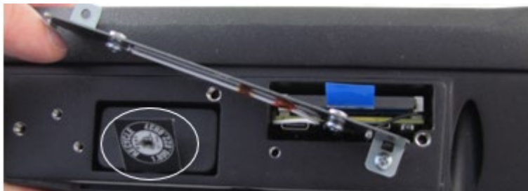
Fig. 15-7: Inserted battery pack
