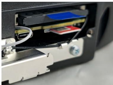
Fig. 11-2: SIM-card-slot under the antenna cap (with Taoglas antenna)
