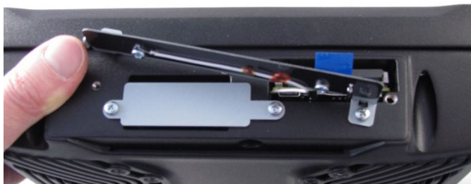
Fig. 15-4: Opened WLAN Diversity Antenna
