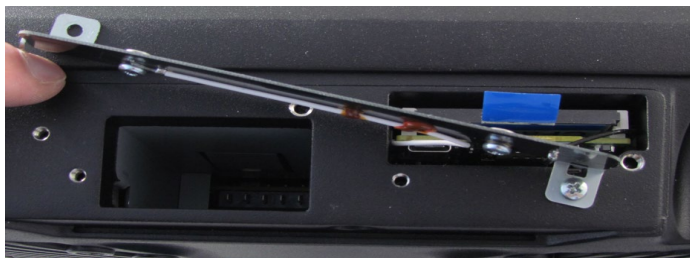
Fig. 15-6: Opened battery compartment
