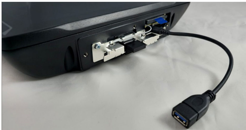
Fig. 7-26: Connected adapter to USB Type-C Service Port (with Taoglas antenna)
